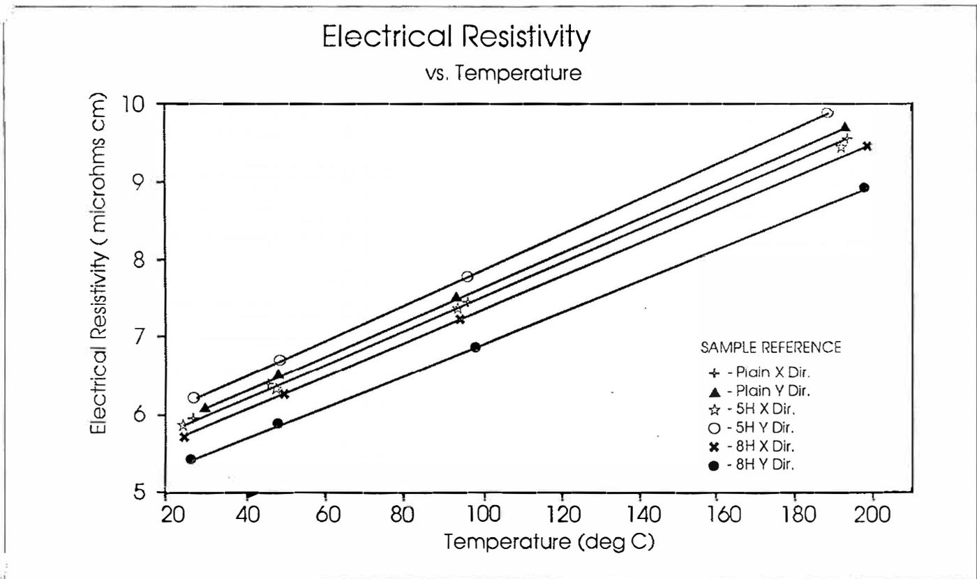
Figure 2. Effect of temperature on electrical resistivity
