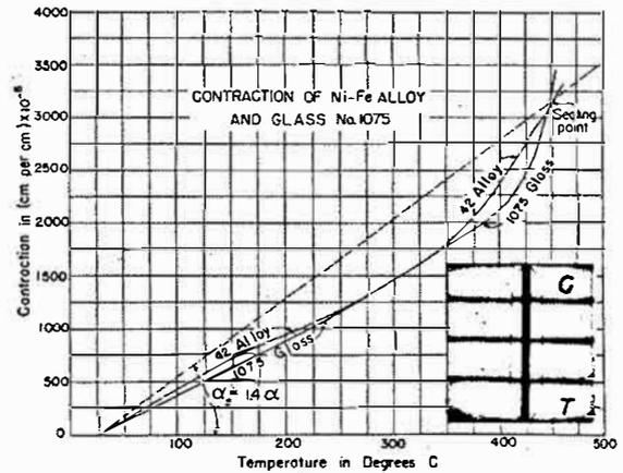
FIG. 10. Thermal expansion curves of 42 alloy and 1075 glass, and photoelastic stress pattern of a seal between them. Absence of stress in the seal is shown by the straightness of the interference lines crossing it.
