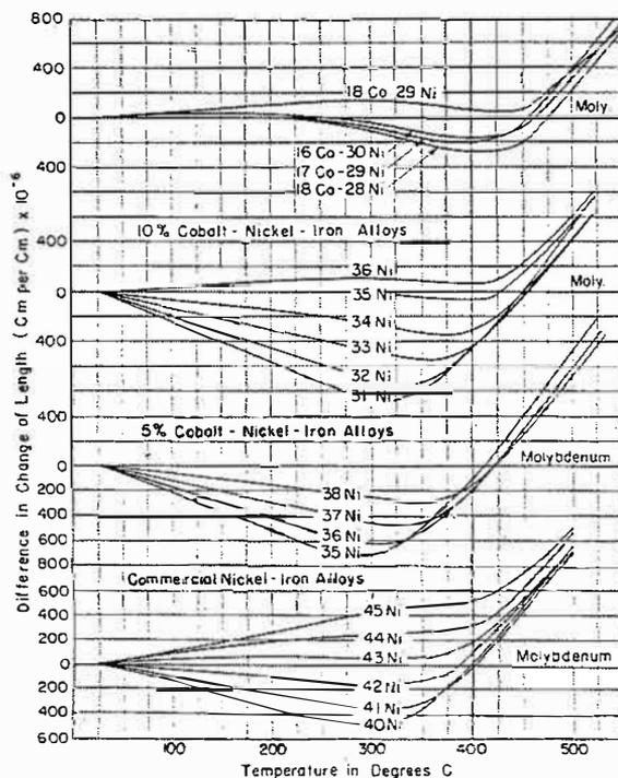
FIG. 1. Thermal expansion of iron-nickel-cobalt alloys, compared to molybdenum.
