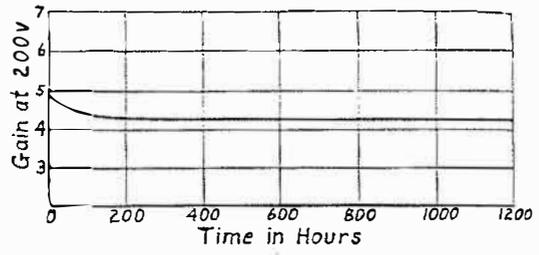
FIG. 4. Alloy activated for maximum stable gain.
