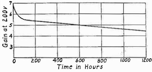
FIG. 3. Alloy activated for maximum initial gain.
