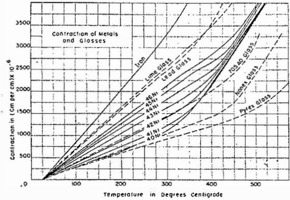
FIG. 9. Thermal expansion of iron-nickel alloys. The expansion curves of the common commercial glasses are shown for comparison.
