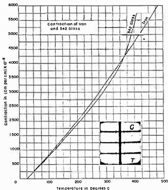
FIG. 12. Thermal expansions of 542 glass and iron, and photoelastic stress pattern of a seal between them.
