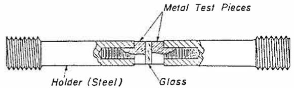
FIG. 13. Form of seal used for testing the strength of bond between metal and glass. The studs, with the glass between them, are screwed into the jaws of a steel-testing machine.
