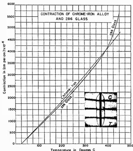
FIG. 11. Thermal expansions of 286 glass and 26 chrome-iron, and photoelastic stress pattern of a seal between them. Absence of stress is shown by the straightness of the dark lines crossing the seal.
