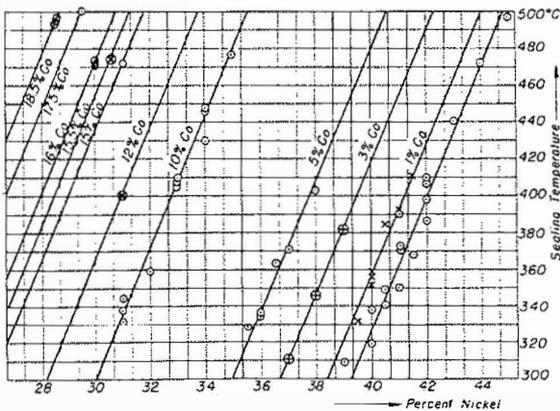
FIG. 3. Sealing temperature of iron-nickel-cobalt alloys as function of nickel and cobalt content.
