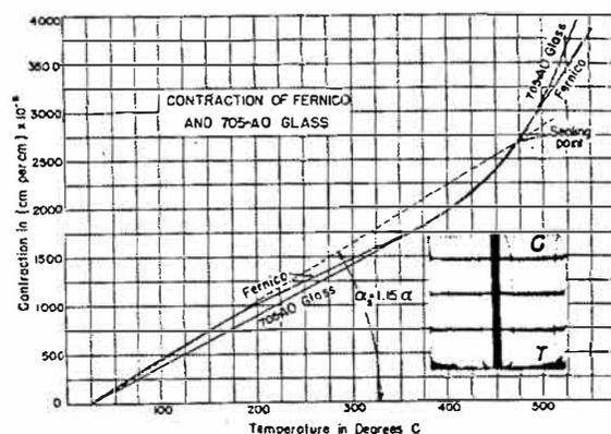
FIG. 2. Thermal contraction of fernico and 705-AO glass. The insert shows the stress pattern of a test seal between these materials.
