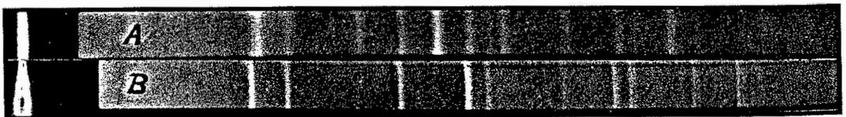
FIG. 8. (A) X-ray diffraction of filings from annealed fernico rod. The body-centered lattice proves transformation to  $\alpha$  phase caused by plastic deformation. (B) Pattern of same filings after 5 min. anneal in  $\text{H}_2$  at  $900^\circ\text{C}$ , showing restoration of  $\gamma$  phase.
