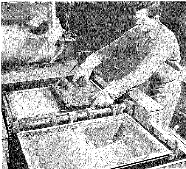
Figure H-34. As the right half of the shell machine is returned to its place, the stripper pins are depressed causing them to push up against the hardened shell and strip it away from the pattern. The shell is then removed from the machine and placed on an adjacent work table. Each machine cycle produces both halves of a shell which when glued together will make a complete mold.
