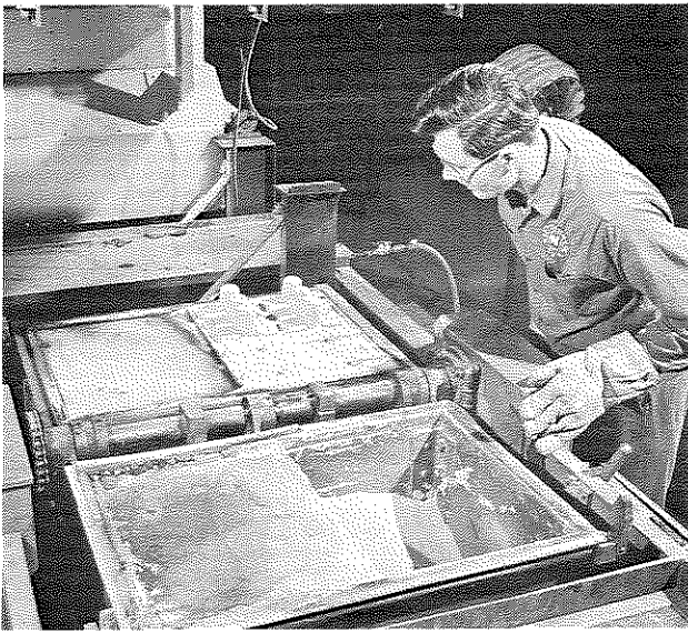
Figure H-33. The sand contains a binder that is heat responsive. Thus when the sand and pattern come in contact, the heat from the pattern is sufficient to bond a thin layer of sand to it as shown here. A flame torch is then used to provide the additional heat needed to harden the sand layer completely.
