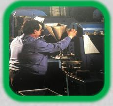
Dedicated to small and medium sized parts where powder is fed automatically into the mold.
