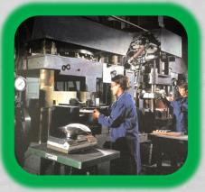
Hand-fed presses are used to produce larger parts. Press tonnage runs from 100-1,000 tons (and higher).
