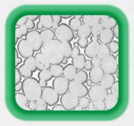
The process of producing Tungsten alloys is termed — **LIQUID PHASE SINTERING.** At the final sintering temperature, the Nickel/Iron or Nickel/Copper powders melt, causing the Tungsten particles to dissolve into solution. Upon cooling, the excess Tungsten nucleates as spherical particles (grey spheres) surrounded by Tungsten — Nickel — Iron alloy (white areas).
